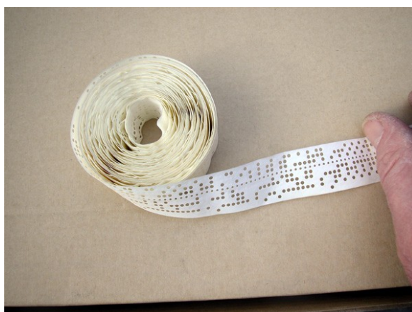
Small reel of 8-hole paper tape: some reels were enormous!
